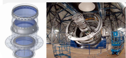
Wide-field Corrector with 2.5s degree diameter field-of-view for the VISTA telescope.
