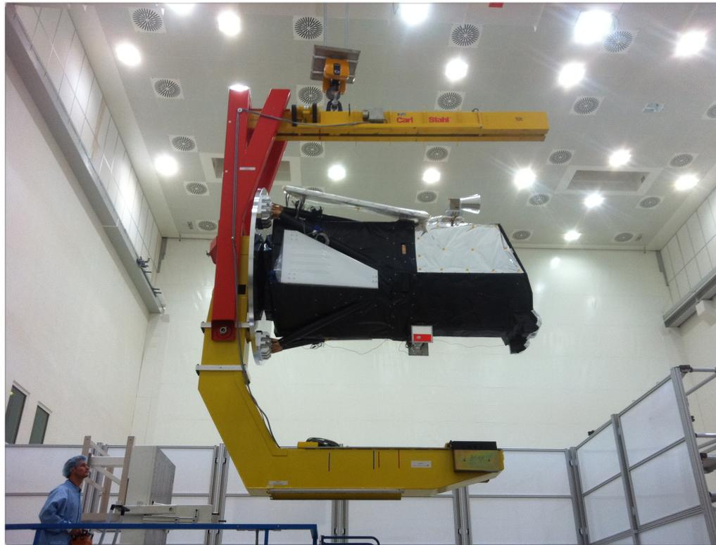
*eROSITA at the space testing facility IABG during mass measurement.*
